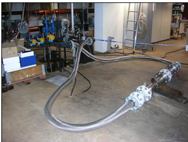
Figure 2. Experimental setup during the high temperature investigations. The VoS-meter was connected to the high temperature test rig via two metal hoses. Two reference sensors were mounted in the setup, one single Pt-100 placed closed to the pump and the Tarray placed downstream the VoS-meter.
