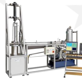
OM2 (Low-flow liquid calibrator)
